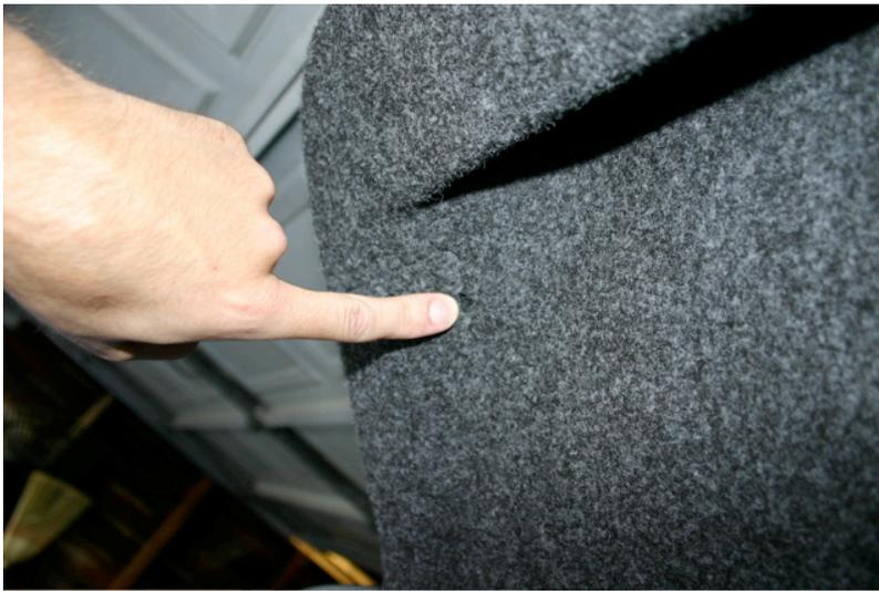
To remove the trunk lights locate the small hole in the trunk liner and insert a screwdriver to pull it loose.
